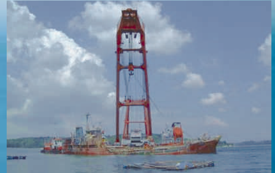
The Endah Lestari, being uprighted and lifted by a floating crane.
