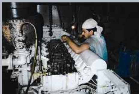
The Haris, receiving preservation treatment after the engine room was flooded.
