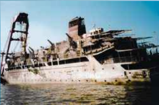
The Leuser, during pumping and refloating operations.
